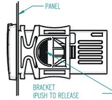
Instrument XR30CX shall be mounted on vertical panel, in a 29x71 mm hole, and fixed using the special bracket supplied. The temperature range allowed for correct operation is 0-60 °C. Avoid places subject to strong vibrations, corrosive gases, excessive dirt or humidity. The same recommendations apply to probes. Let air circulate by the cooling holes.
