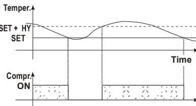
In case of fault in the thermostat probe the start and stop of the compressor are timed through parameters **Con** and **CoF**.
