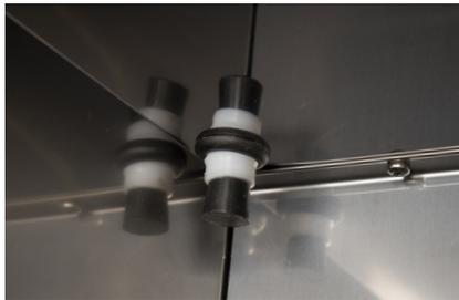
Porthole for external temp. sensors
