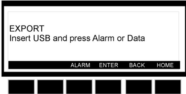
5. Select ALARM or DATA, the controller starts sending data to the pen drive, when the export is finished the message: **EXPORT - Copy completed** is displayed.
