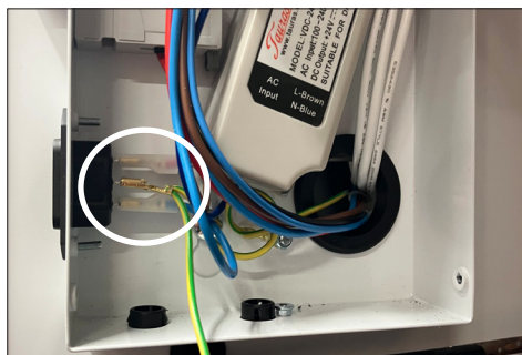
4. Loosen the ground wire from the plug
