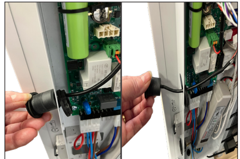
4. Remove the USB C outlet connector, replace with new one
