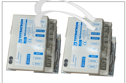
7. Exchange the wires from the old ECU to the new.
