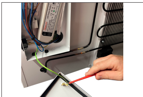
3. Loosen the ground wire from the lid
