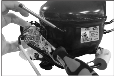
4. Use a screwdriver to loosen the starting device from socket and pull.
