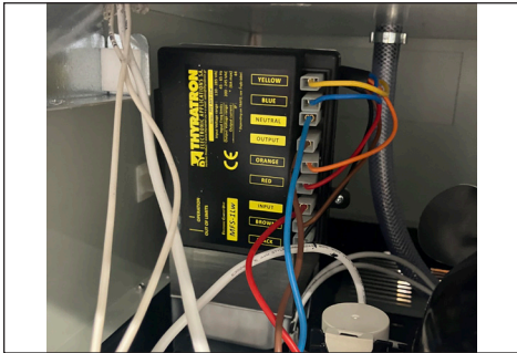
3. Remove the wires by pulling on the terminal housing, not on the wires.
