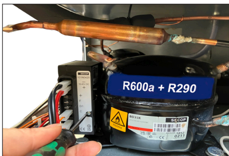
2. Loosen the screw a couple of turns.
