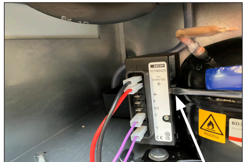
3. Place a screwdriver in the small vent in the plastic cover.
