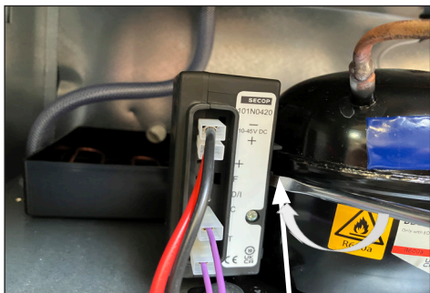
4. Unclick plastic cover/starter g device from compressor bracket
