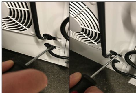
2. push the rubber ring in carefully
