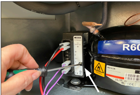
2. Loosen the screw a couple of turns.
