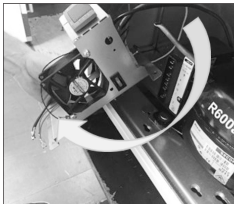
3. Gently pull out the thermostat bracket, by tilting out from bottom.
