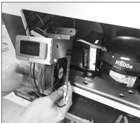
3. Gently pull out the thermostat bracket, by tilting out from bottom.
