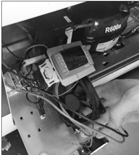
4. Push clip on left and right side and pull out thermostat.
