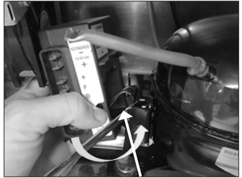
4. Use a screwdriver to disconnect the socket from compressor.
