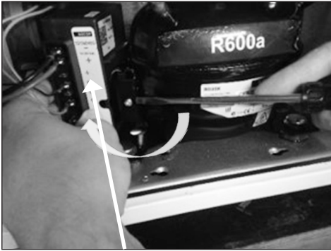
3. Unclick plastic cover/starting device from compressor bracket.
