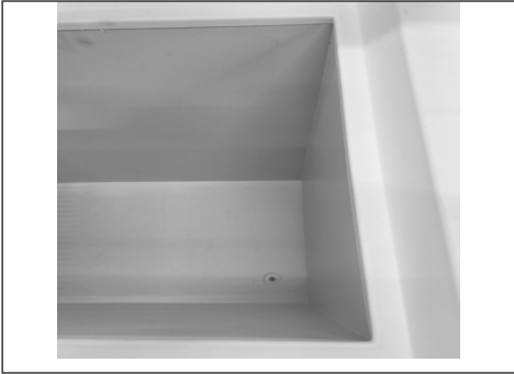
1. The drain is in the bottom
