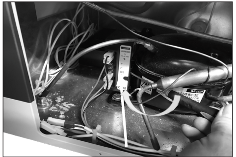
4. Unclick plastic cover/starting device from compressor bracket
