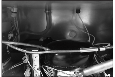
7. IMPORTANT! When re-mounting the new thermometer make sure the wire sealing plug is placed properly
