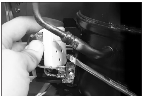
5. Starting device loose from socket
