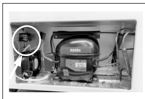
The thermostat is placed in the left corner of the compressor compartment on the terminal bracket
