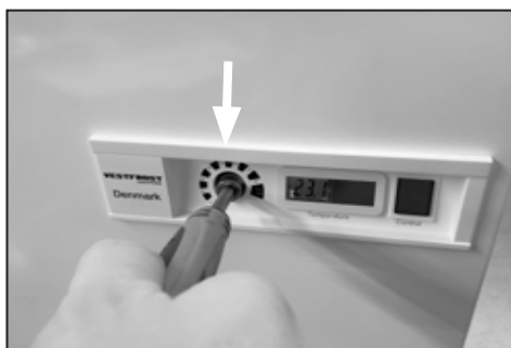
Use a socket wrench Size 13mm to unscrew the fixing nut
