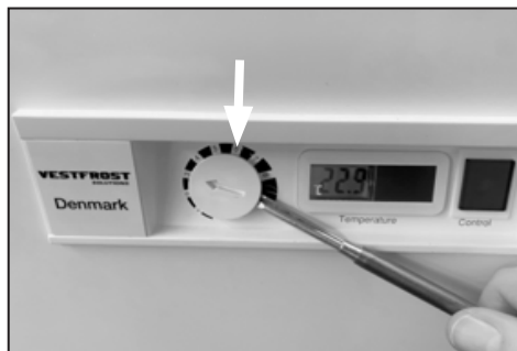
Use a screwdriver to gently remove the plastic cover dial.
