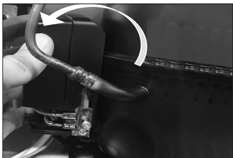
3. Pull the cover back to loosen.
