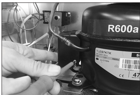
1. Dismount the cover for starting device by loosen the phillips screw.
