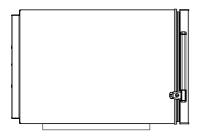
To avoid damage place a soft bedding under the unit (e.g. the packaging) and then tip the unit.
