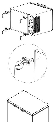
To attach the wheels, use the 8-mm hex key to tighten the screws.
