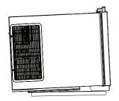
To avoid damage place a soft bedding under the unit (e.g. the packaging) and then tip the unit.
