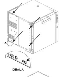
Note: Wheel mounting holes are different from the holes used for the feet
