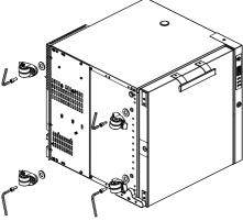
To attach the wheels, use the 8-mm hex key to tighten the screws
