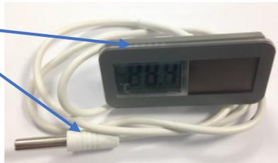
8: **IMPORTANT!** When re-mounting the new thermometer remember to properly seal the wire feedthrough
