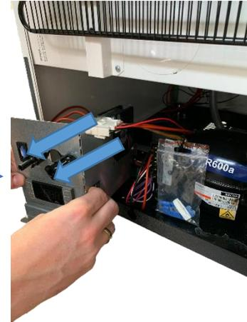
3. Flip it around to allow easy access to thermostat
