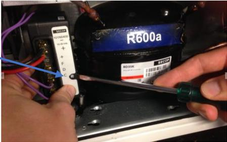
3: Unclick plastic cover/starting device from compressor bracket
