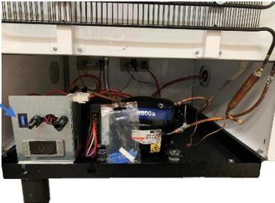
1. Use the small fuse- tool supplied together with spare fuses in the small plastic bag together with appliance or a plier .
