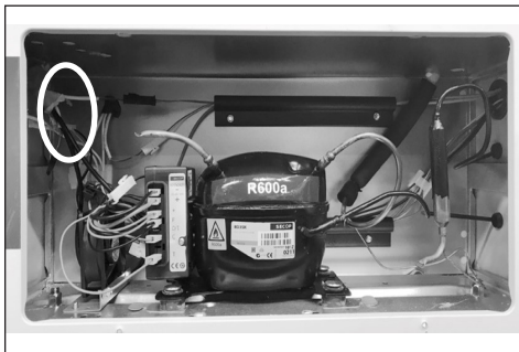
The icebank sensor is placed in the corner
