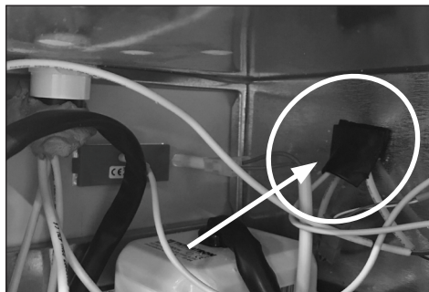
11. IMPORTANT! When re-mounting the new thermometer remember to properly seal the wire feed through.
