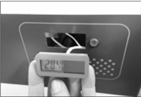
6. Temperature monitor is loose from cabinet.
