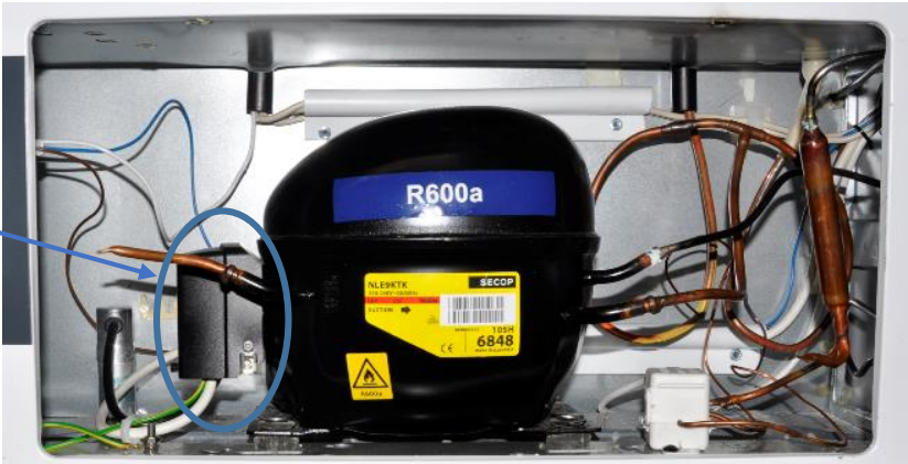
The starting device is mounted on the left side of the compressor
