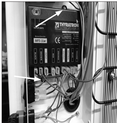
2.Loosen the 2 screws and remove the wires
