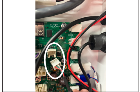
2. Remove the wires.
