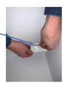
3: Remove sealing kit from wirefeedthroug inside vaccine compartment
