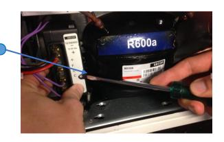
5: Unclick plactic cover/starting device from compressor bracket
