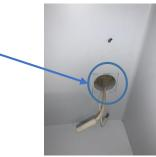
4: Remove sealing kit from wirefeedthroug inside compressor compartment
