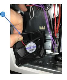
6: Fan can be replaced by new one
