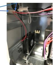
1: Cut the cable tie to release wires
