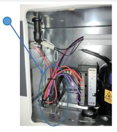
2: Unplug the fan power wires (Black/Red) gently from the terminal using a plier or by hand
