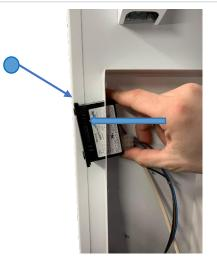
7: Switch the sensor wire plug from old socket to the new
