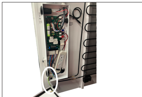
2. Be careful with the lid as the ground wire is attached to the lid
