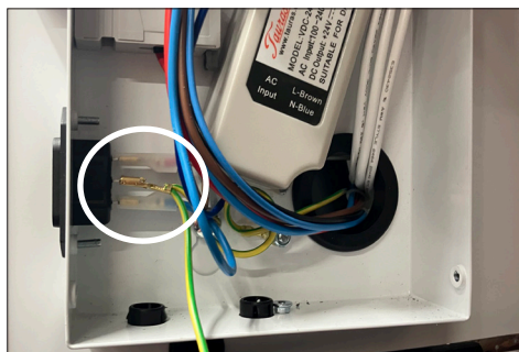
4. Loosen the ground wire from the plug
