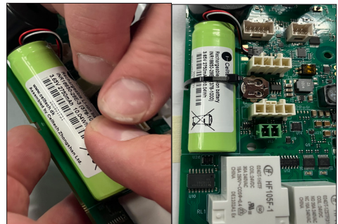
4. The battery has been changes make sure to fasten it again
