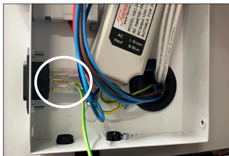
4. Loosen the ground wire from the plug
