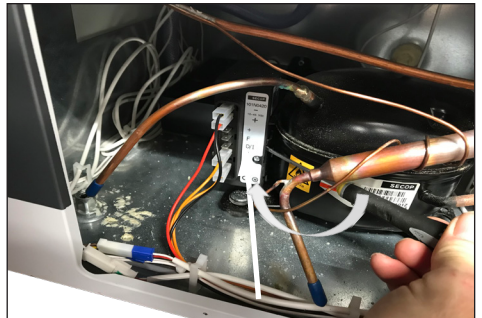
4. Unclick plastic cover/starting device from compressor bracket
