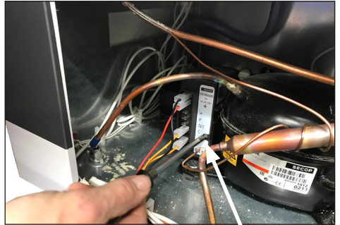
2. Loosen the screw a couple of turns.
