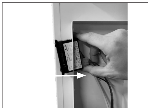
8. Place the thermostat back in place of the junction box
