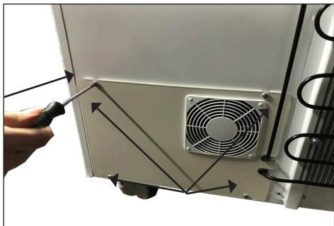
1. Use a screwdriver to loosen all 4 screws.
