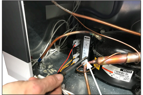
2. Loosen the screw a couple of turns.
