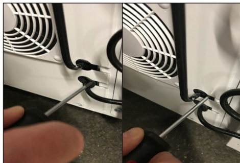
2. push the rubber ring in carefully
