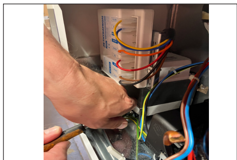
3. Loosen the screws from voltage stabilizer controller/transformer bracket
