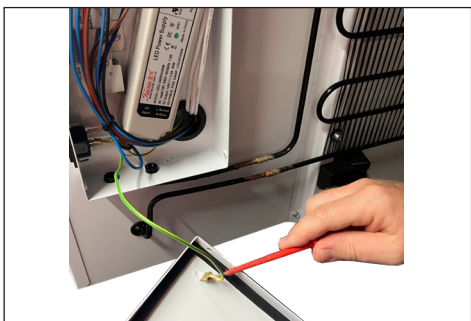
3. Loosen the ground wire from the lid
