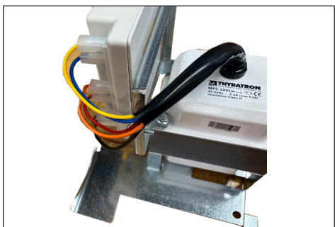
5. Untighten the 8mm bolt connecting the stabilizer controller to the bracket
