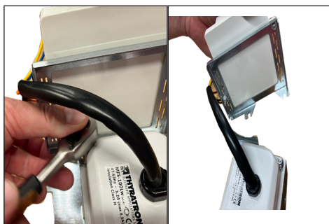
6. Take apart the controller and transformer.
