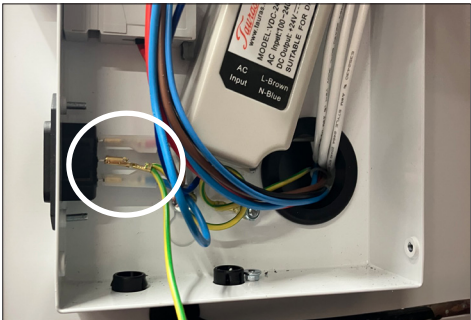
4. Loosen the ground wire from the plug
