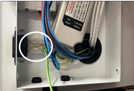
4. Loosen the ground wire from the plug
