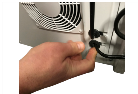
7. When the grid is put back in place, be suer that the rubber ring is placed correctly
