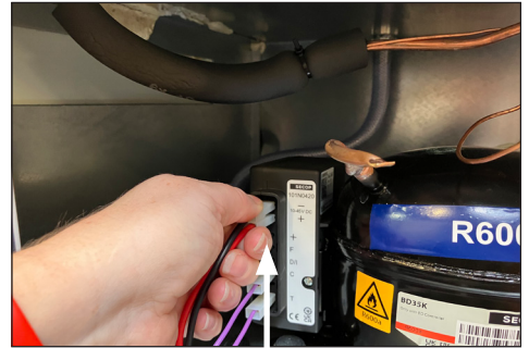
1. Dismount the 4 wires from ECU. Grab the wire socket and pull gently.
