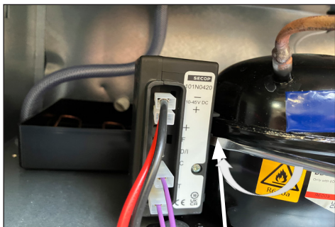
4. Unclick plastic cover/starting device from compressor bracket
