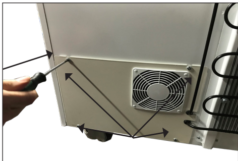
1. Use a screwdriver to loosen all 4 screws.
