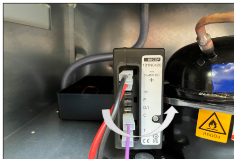
5. Use a screwdriver to disconnect the socket from compressor.
