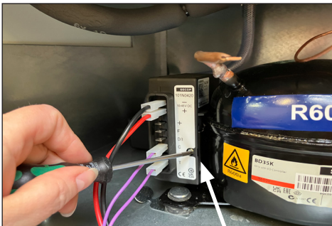
2. Loosen the screw a couple of turns.
