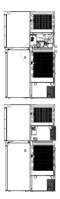
Place the bracket between the two units
