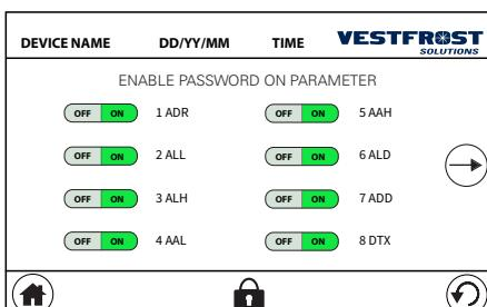
By accessing the parameter password page, it is possible to select on which parameters the service code is enabled for modification (on) and on which parameters the modification will not ask for the service code (off):
