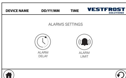
where it is possible to access the settings page of the alarm signal delay and snooze time (silencing time of the acoustic signal when, in the presence of an alarm, the snooze button is selected):
